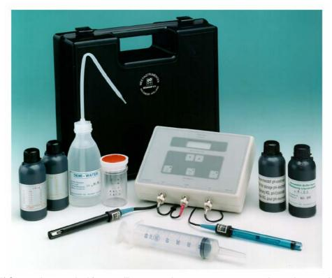
This EC/pH/°C-meter has standard features like; automatic temperature compensation and automatic calibration. Is supplied complete in a rugged carrying case included accessories for water- and soil samples.
