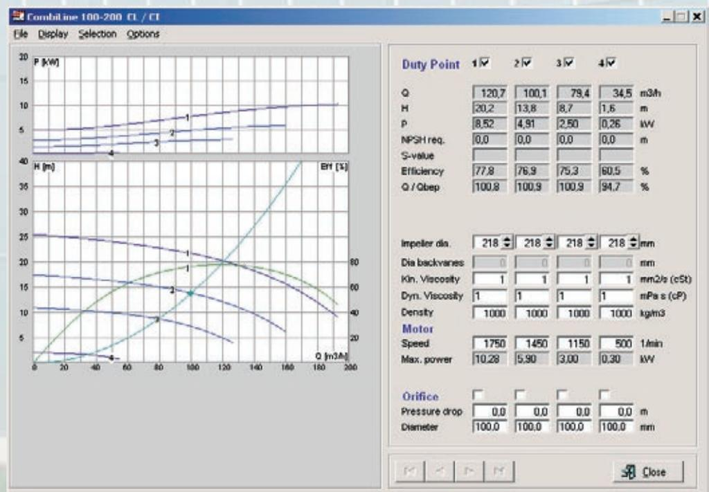
**Example:** CL 100-200 with 7.5 kW motor 50 Hz (8.6 kW at 60 Hz).
