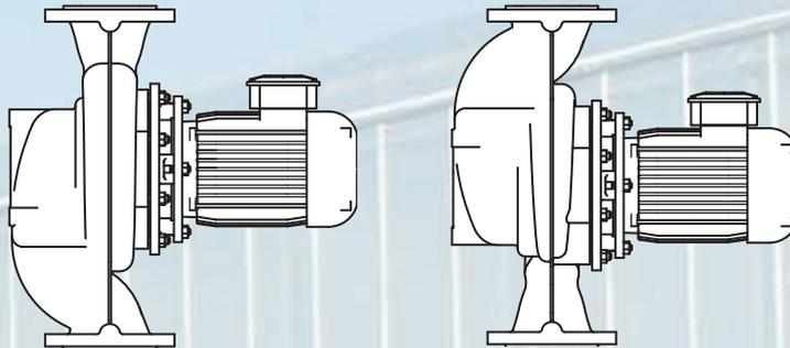
Horizontal, with motor in vertical position. If necessary, the pump can be mounted on a base plate and foundation to avoid pump loads to the pipe work in case of large weighty pump types.
